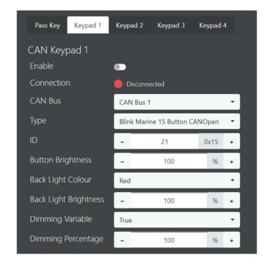
is equal to True. This is useful for night time operation. The Dimming Percentage is the brightness of the Buttons and Backlight as a percentage of the Button Brightness and Backlight Brightness settings.
