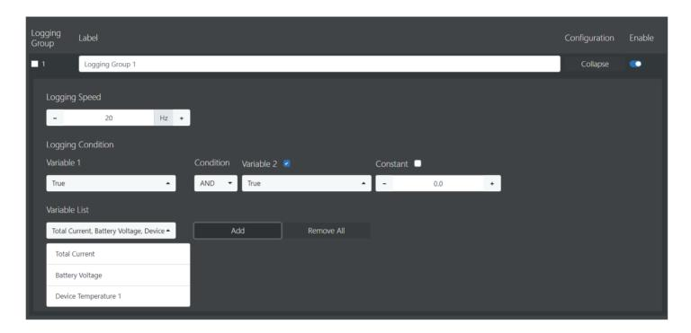
Each Logging Group is responsible for data logging a collection of variables. These variables are logged at the Logging Speed, which can be changed between 1-20Hz. The variables are logged whenever the Logging Condition evaluates to True. In this example, the Logging Condition is set to 'True AND True,' which will mean that the data is continually logged. Variables to log can be selected below.
