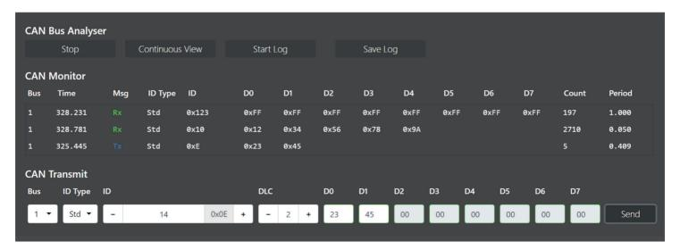
When the CAN Bus Analyser is running, the data can be logged in real time to a CSV file. This data can then be viewed in an external program at a later date. Press Start Log to start a data log. Press Stop Log to stop logging CAN data. Once a data log has been stopped, the user can save the Log to the PC.
