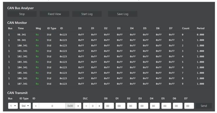
The image below shows the CAN Bus Analyser in Fixed View Mode. In Fixed View Mode, only the latest CAN Bus message with each unique ID is displayed.
