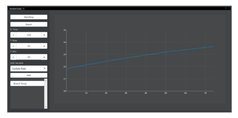
Live data gathering from the PDM can be halted at any moment by pressing the 'Stop' button at the top of the graph window. With the live graphing of variables stopped, the buttons at the top of the graph may be used to zoom in/out, save images of the graph, or to export the graph as a .csv file for viewing on external software. The graph windows can be resized, docked, and tabbed by clicking and dragging on the top of the graphing window.
